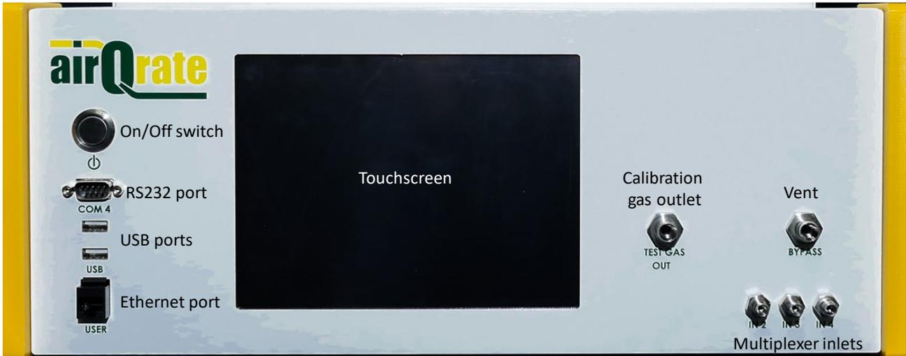
*Figure 2: Front view of the mobile airQrate*
