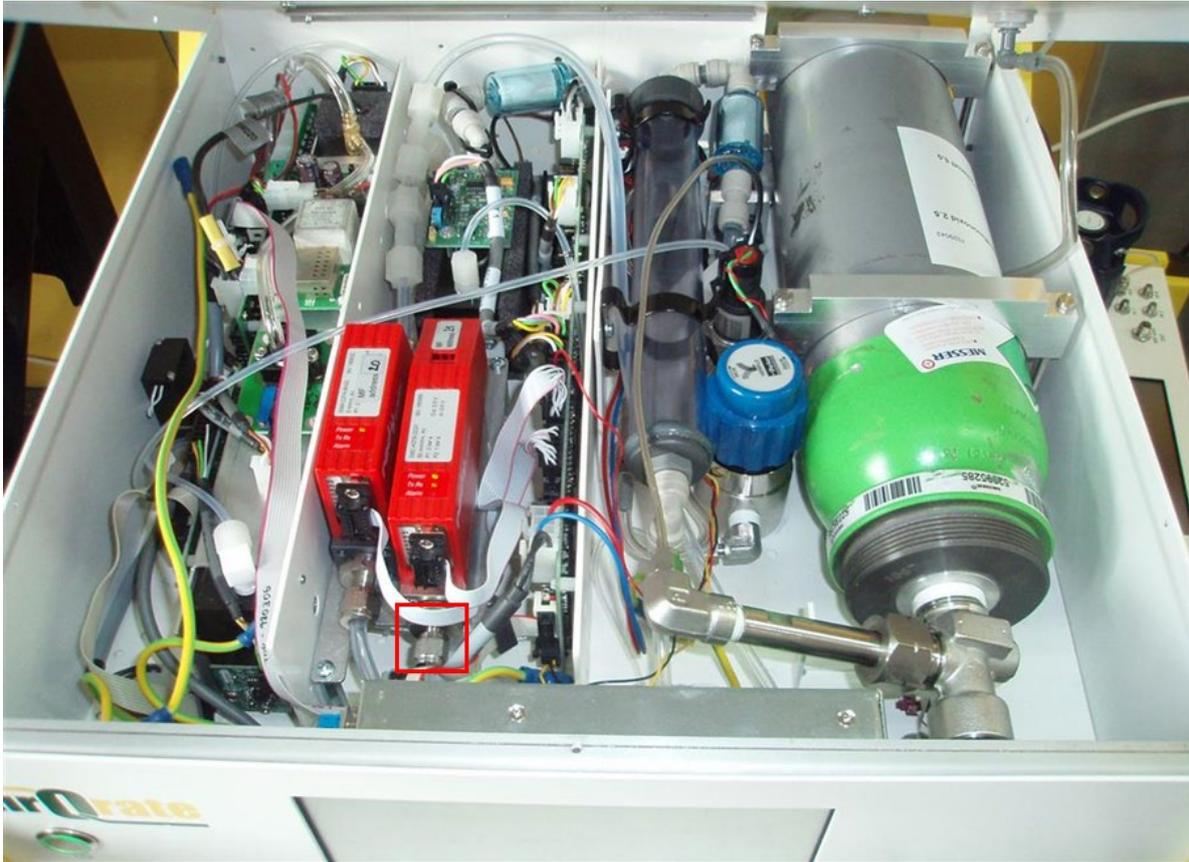
*Figure 6: Purging the high-pressure tubing*
