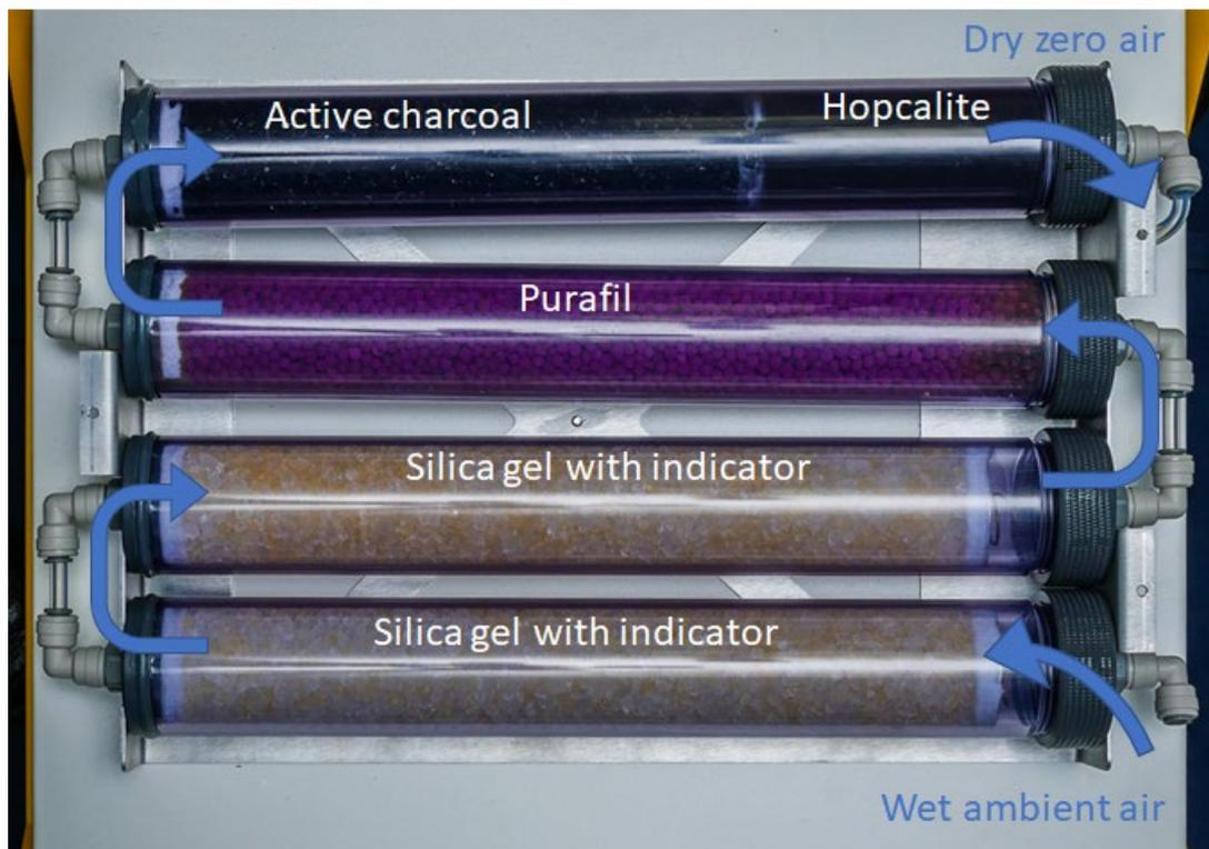
*Figure 41: Cartridges generating zero air*
