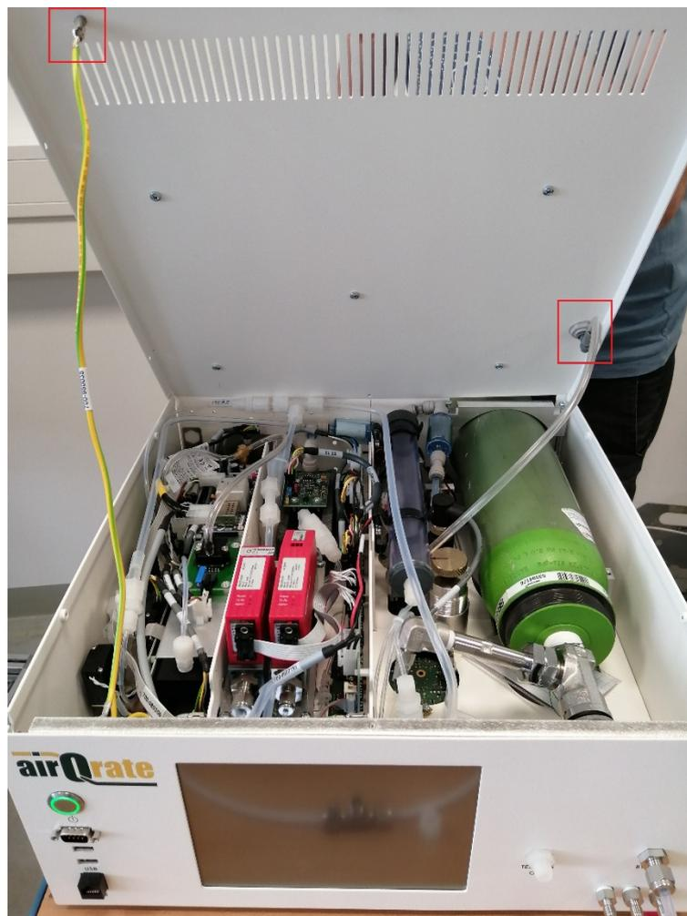
*Figure 4: Removing the cover of the mobile airQrate*
