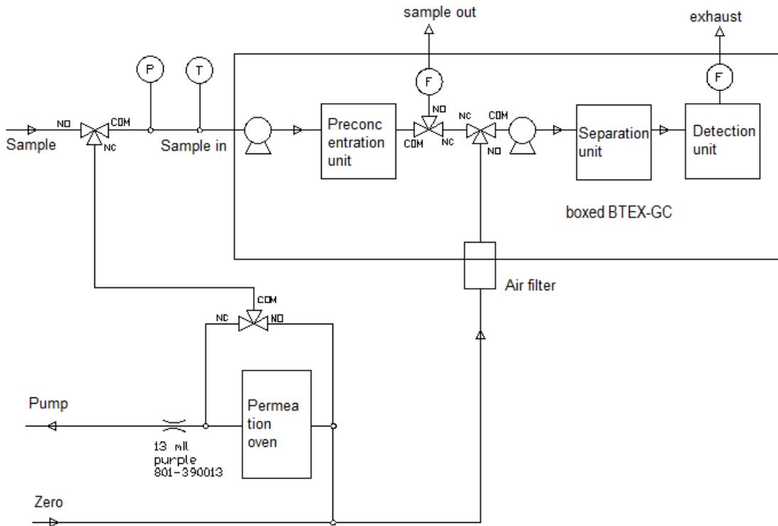
FIGURE 10: FLOW DIAGRAM OF THE BTEX-GC MODULE
