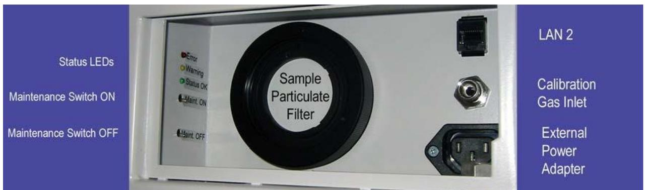
Figure 4.13.: Inside the Maintenance Door of the airpointer
