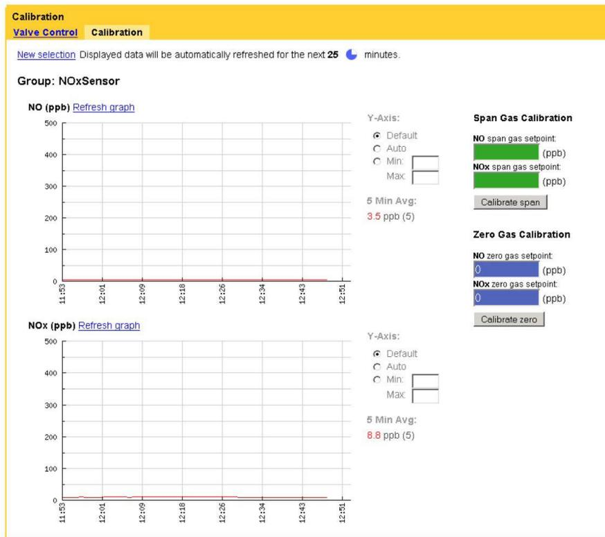
Figure 5.11.: Display of the calibration and input of the setpoints
