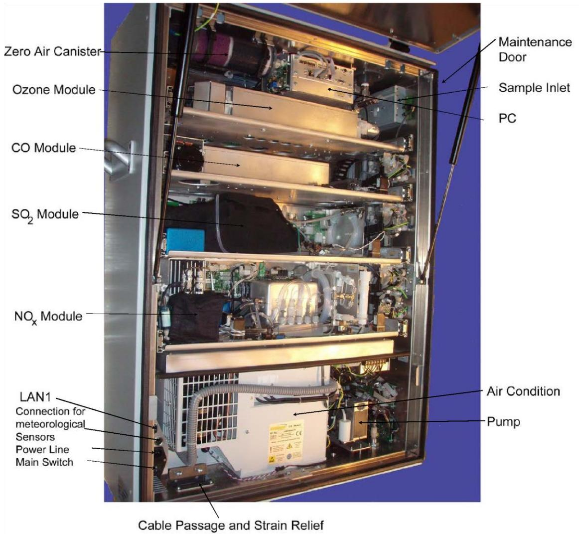
Figure 4.12.: Inside the airpointer with four drawers (4D)
