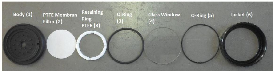
Figure 6.13.: Parts of the Sample Particulate Filter
