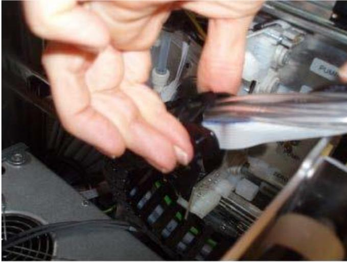
Figure 6.8.: Loose the clamp
