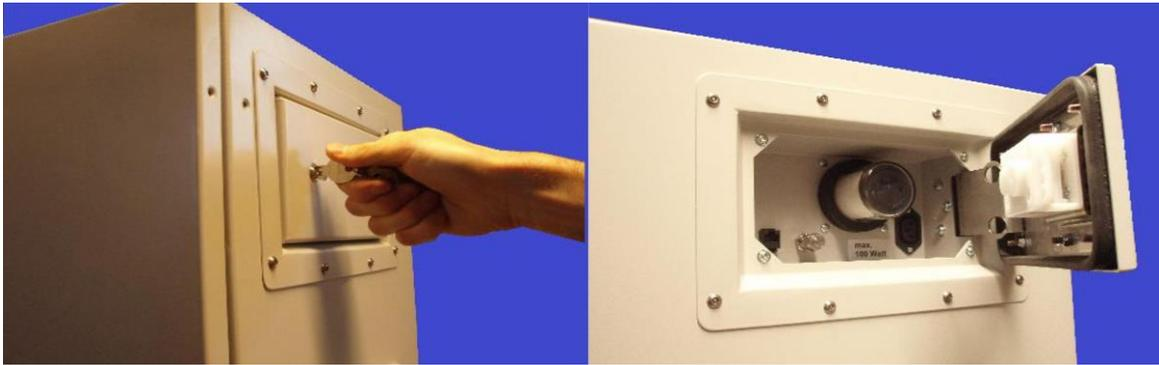
Figure 6.4.: Open and close the maintenance door
