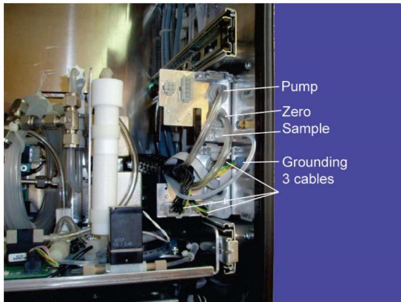
Figure 6.6.: Disconnect the seven connections of the connection chain.
