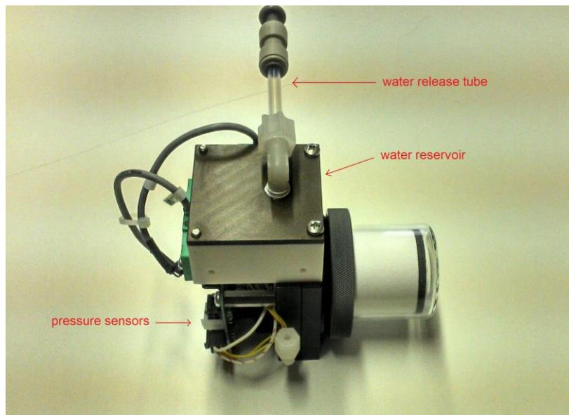
Figure 6.15.: An Extended Lifetime Filter with both options
