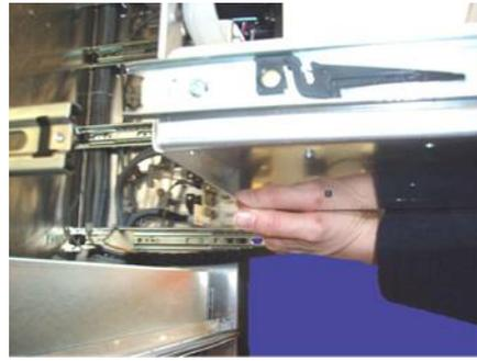
Figure 6.11.: Hold the module with one arm near the drawers
