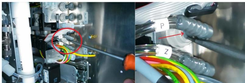
Figure 6.7.: Pushing down the grey ring with a screwdriver
