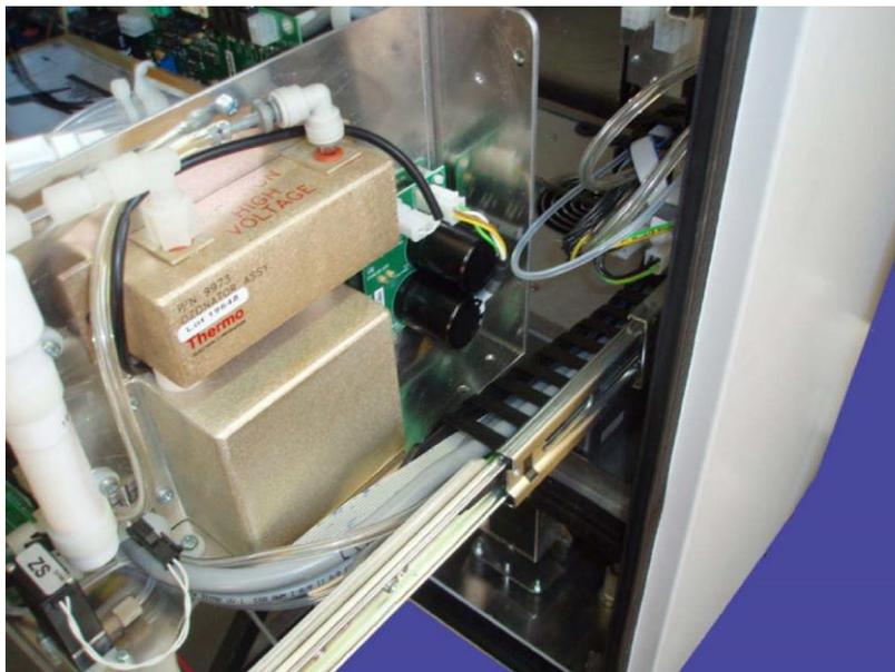
Figure 6.5.: Push and pull the module on both sides simultaneously
