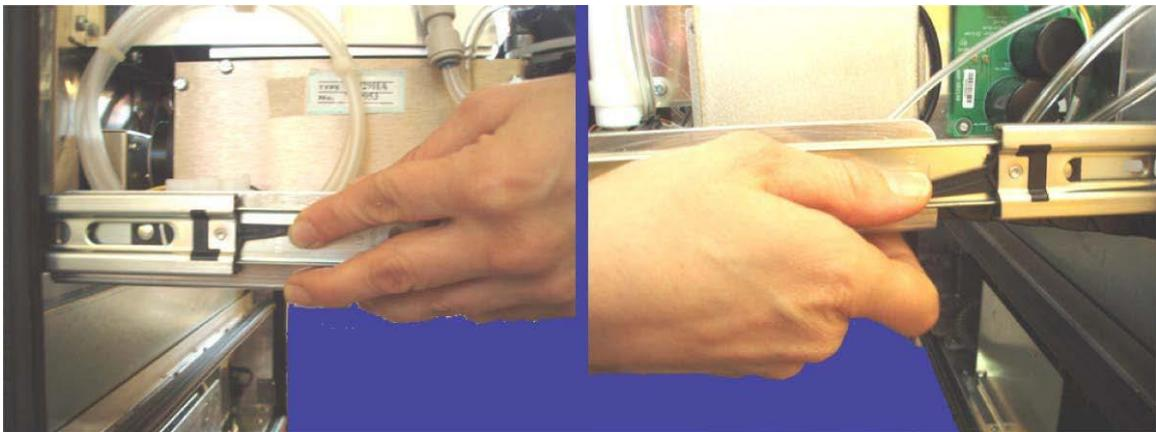
Figure 6.9.: Press the small levers in both drawers up (left) or down (right).
