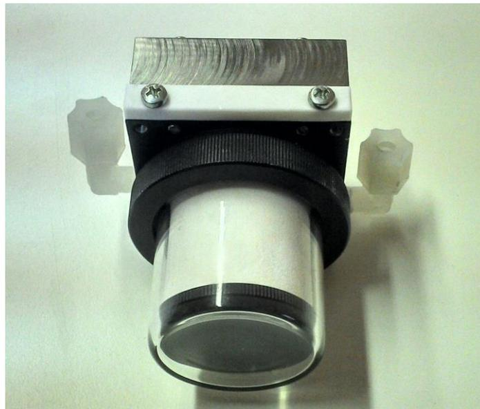
Figure 6.14.: The basic Extended Lifetime Filter
